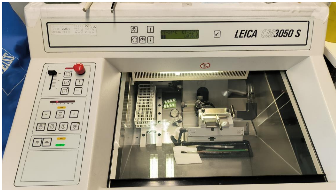
Figure 13; Cryostat. Photo of the cryostat showing: the console (which allows setting adjustments), the cryochamber, and, at the center, the microtome. It is also possible to notice the presence of tools such as brushes and tweezers, very useful during cutting to facilitate the orientation and adhesion of the sections on the slide.
