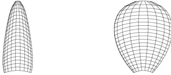
Figure 14: Grid for DC4381 Propeller, No Skew-No skew-induced rake. M_{sp} \times N_{ch} = 20 \times 10
