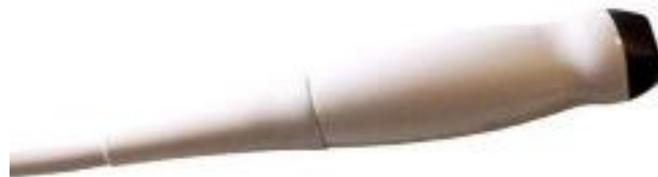
*Figura 8 - sonda phased array P 2-9*
