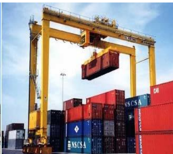
Fig. 2.8 – RTG (rubber tyre gantry crane)
