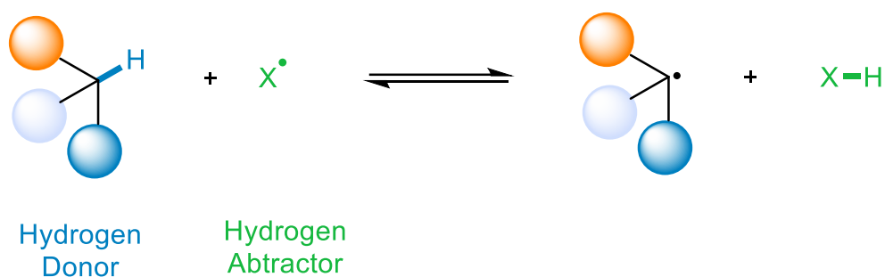
SCHEME 2.1 "Homolytic Cleavage of a C-H Bond via a Hydrogen Atom Transfer step"
