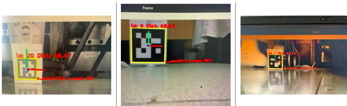
Figure 4.1: camera pose estimation values in real experiments, from left to right the expected values were x=120, y=0 ; x=51, y=65 ; x=31, y=-30 .
