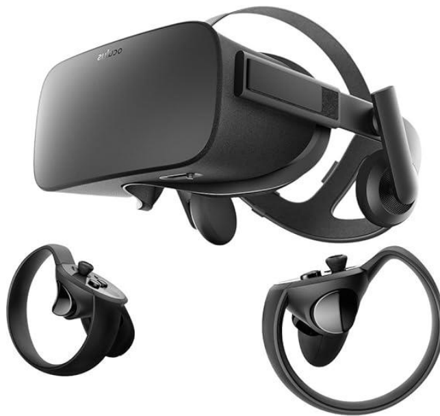
Figure 11 Oculus rift HMD and its hand tracking controllers
