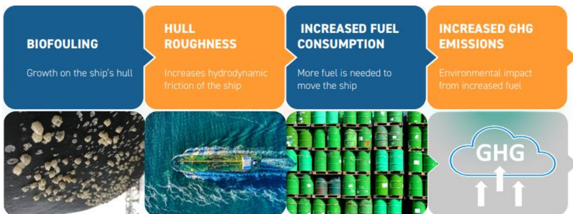
Figure I.1 The ship hull biofouling penalty
