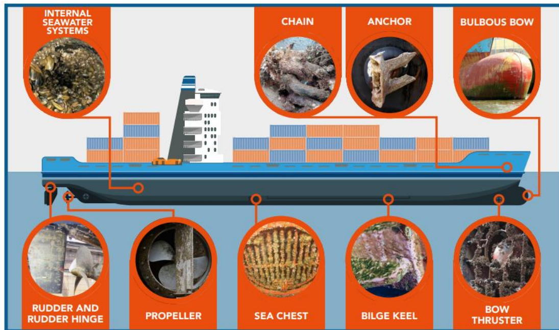
Figure I.7 Typical niche areas on a merchant vessel
