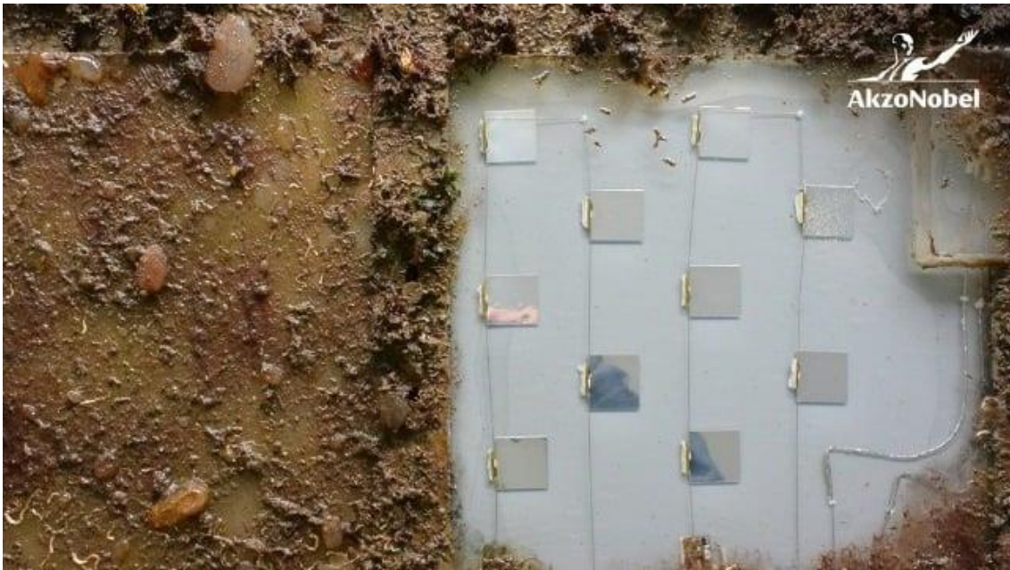
Figure II.7 UVC LEDs testing panel
