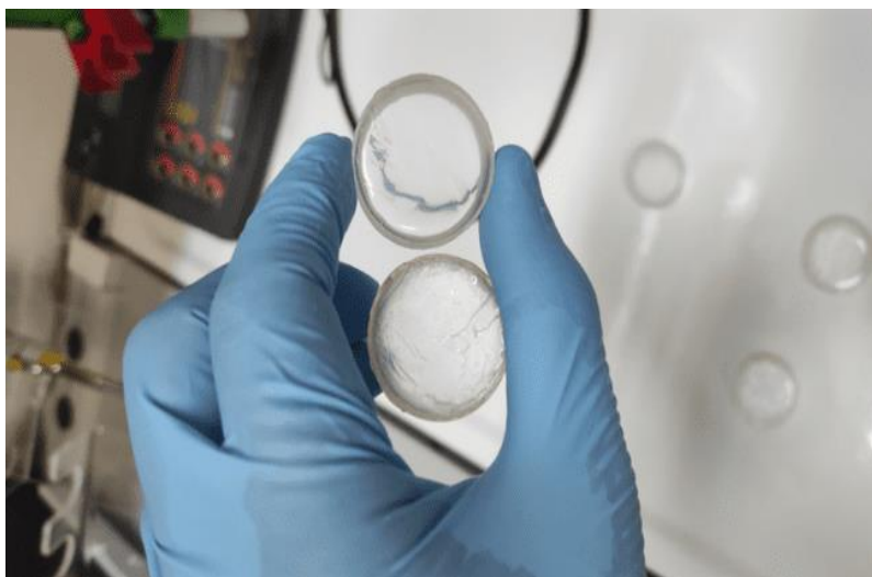
Figure 3.7 Polydimethylsiloxane PDMS lids.
