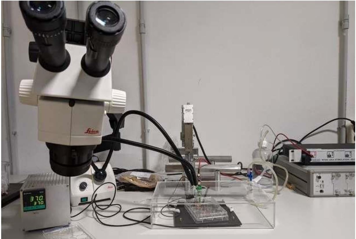
Figure A.2 Acquisition setup with complete Neuronexus probe
