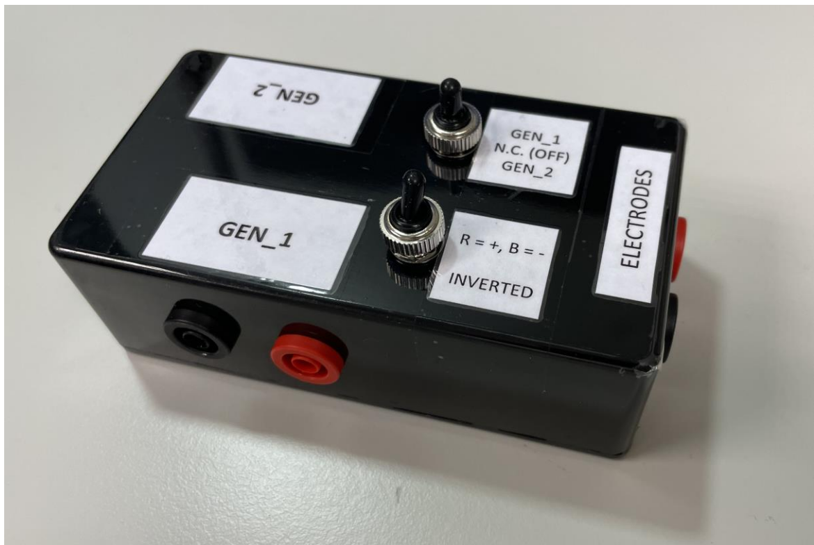
Figure 13: The switchbox used for easy changing of polarity and generator source.
