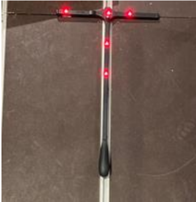
Figure 2.3: World Reference Frame set-up with the Vicon calibration wand.
