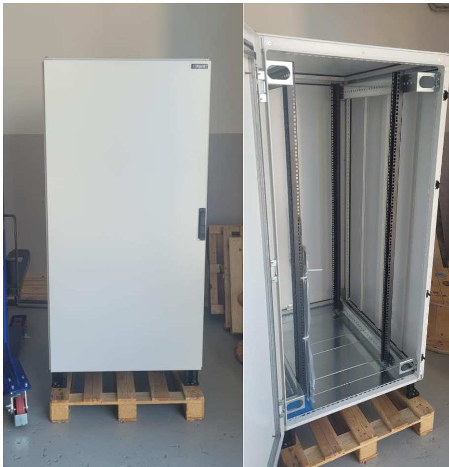
Figure 24. The industrial rack that holds everything together
