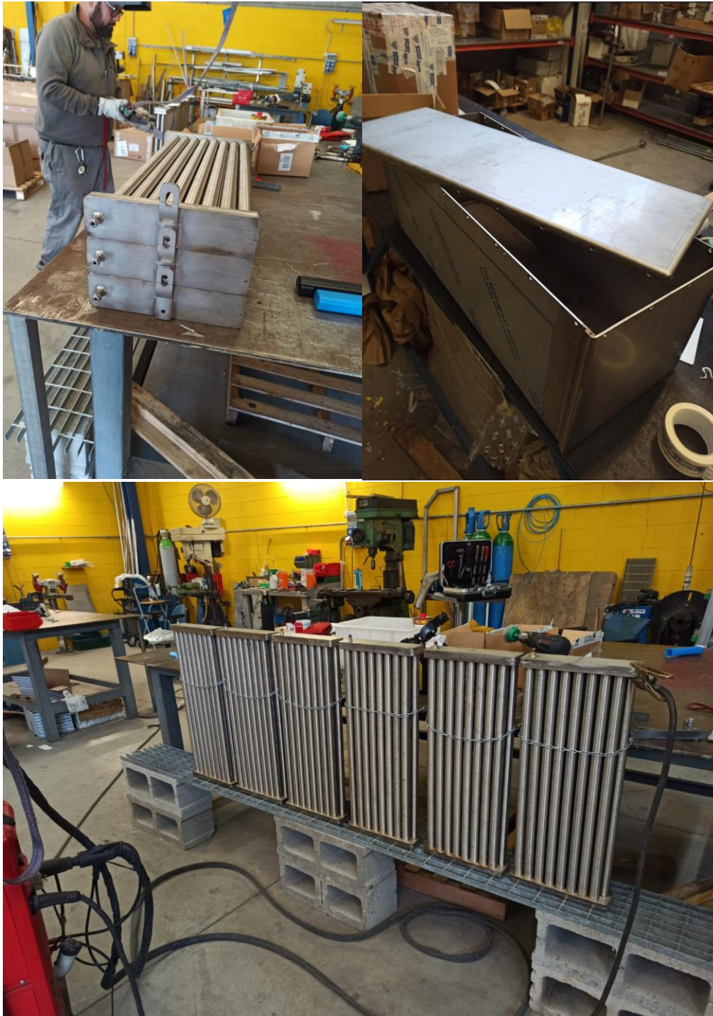
Figure 15. The hydride bank being assembled. Clockwise: the modules stacked; the water vessel; and the soldering of the modules.
