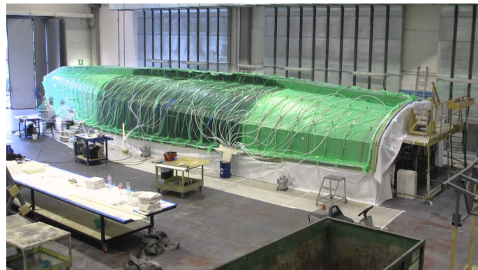
Figure 1.6: Resin Infusion of a carbon fiber IMOCA hull in Persico shipyard
