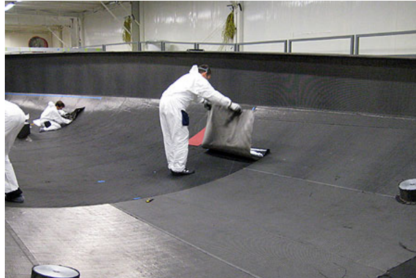
Figure 1.7: Pre-Preg carbon fiber sheets being laid out on a hull mold
