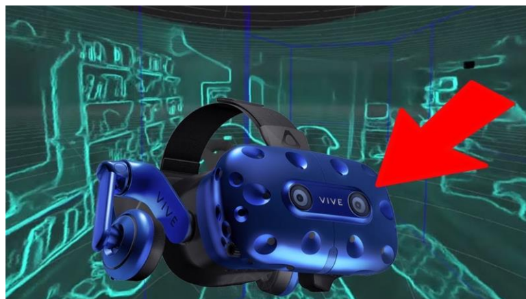
Figure 2.2 The camera placed on the frontal face of the HTC Vive Pro.
