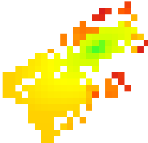
Figure 4-18: Configuration 4 - Map of expected precisions in Z direction (in meters) obtained with rigorous method
