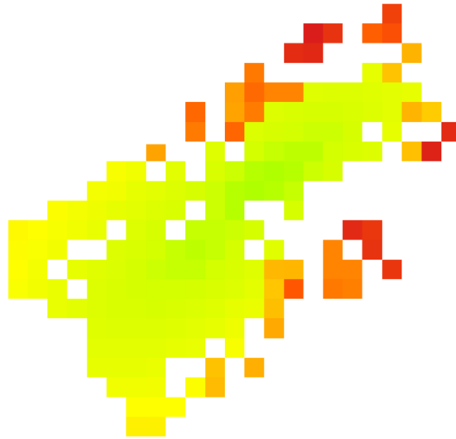
Figure 4-22: Configuration 5 - Map of expected precisions in Z direction (in meters) obtained with rigorous method
