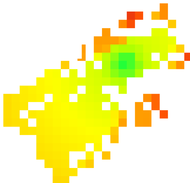
Figure 4-17: Configuration 4 - Map of expected precisions in Y direction (in meters) obtained with rigorous method
