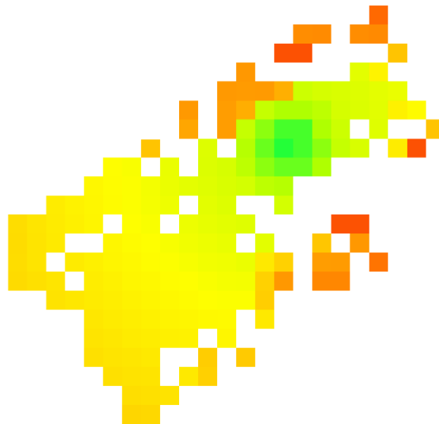
Figure 4-16: Configuration 4 - Map of expected precisions in X direction (in meters) obtained with rigorous method
