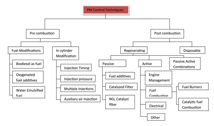
Figure 1-1: Particulate matter emission control techniques
