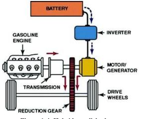
Figure 1-4: Hybrid parallel scheme
