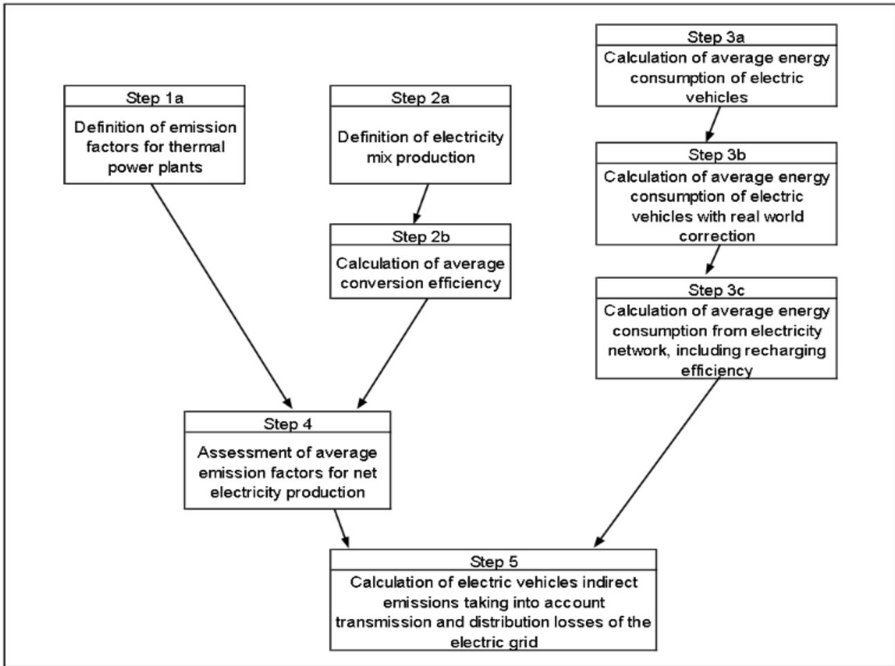
Figure 2-4: Procedure for evaluating the Indirect emission factors for EV
