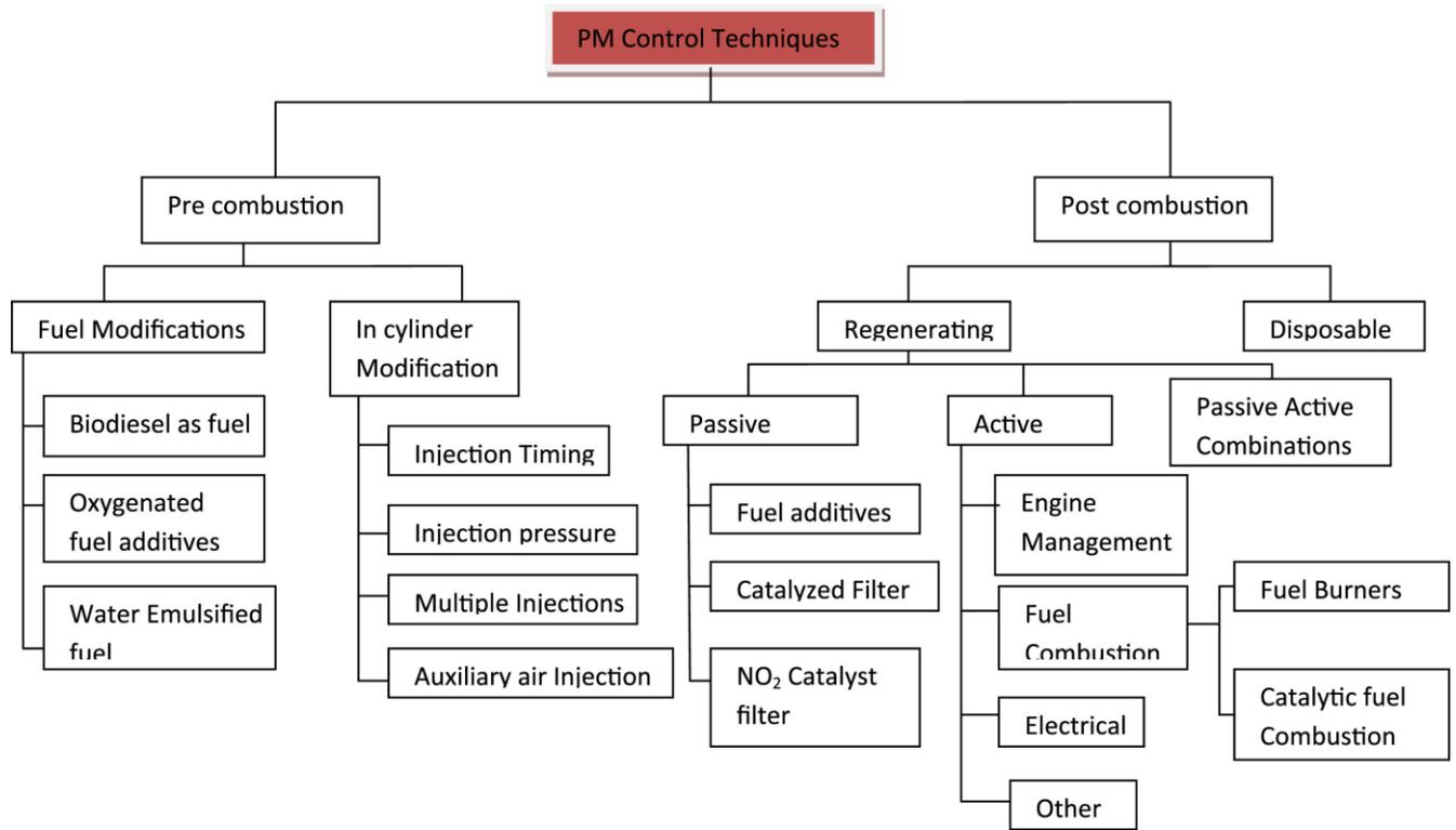
Figure 1-1: Particulate matter emission control techniques
