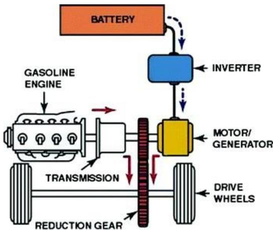
Figure 1-4: Hybrid parallel scheme
