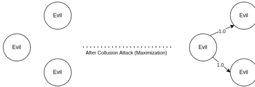
Figure 3.1: Network state evolution during a Collusion Attack operating within the maximization paradigm. By forcing a maximum transaction outcome ( O = 1.0 ), malicious nodes maximize their mutual trust to reduce the risk of being isolated inside the network and increase their chances of being selected from the trade pool.
