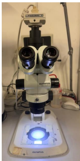
Figura 3.4: stereomicroscopio Olympus SZX7.
