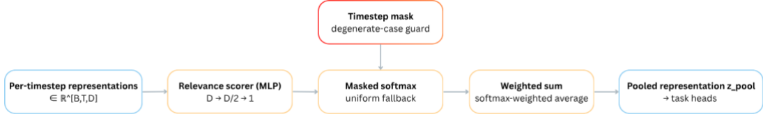
Figure 4. 6 Temporal Attention Pooling. A learned query vector attends over the T per-timestep representations produced by the temporal encoder, yielding a single fixed-size context vector that summarises the full scenario window for downstream classification and regression.
