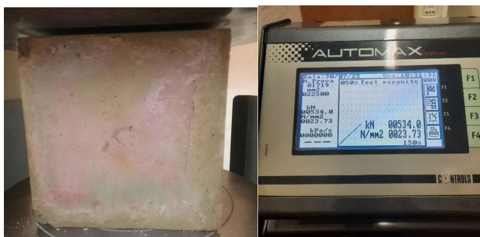
Figure 20. The failure crack pattern of the 90-day specimen.
