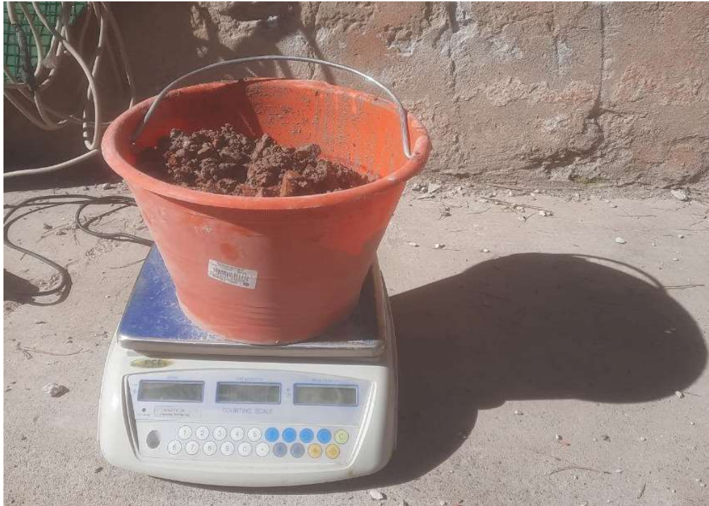
Figure 17. The water is removed, and wet aggregates are weighted
