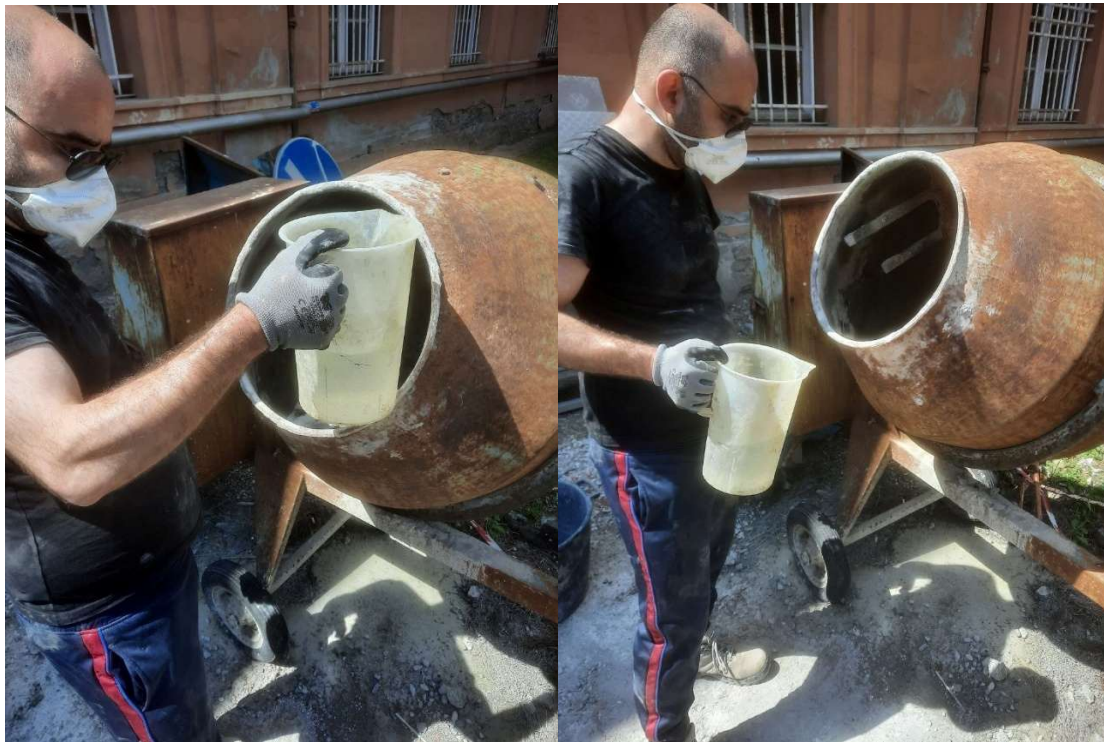
Figure 25. During the preparation of the recycled aggregate concrete, water was added incrementally and carefully to the mixer to achieve the required workability. As shown in the figure, this step was performed manually to ensure better control of the effective water content. The adjustment was necessary because recycled aggregates, particularly mixed debris and broken concrete, exhibited high water absorption, which reduced the amount of free water available for cement hydration. By gradually introducing water, it was possible to compensate for the absorptive behaviour of the aggregates while avoiding an excessive increase in the effective water–cement ratio.
