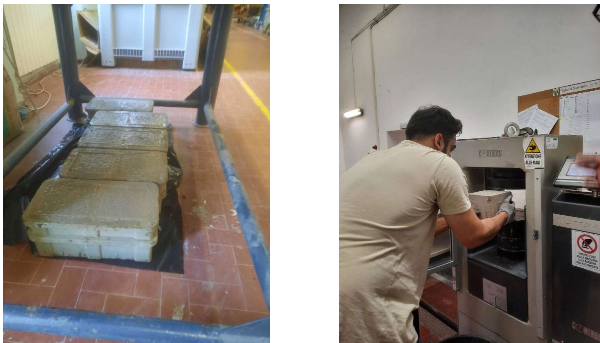
Figure 19. Making the specimens in the framework, extracting them, immersing them in water and finally testing them. All pictures are taken in the laboratory of university of genoa
