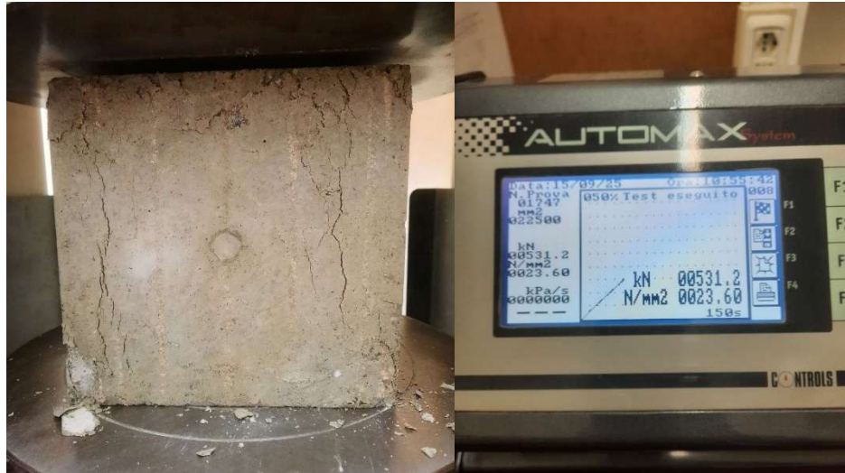
Figure 52. The failure crack pattern of the 90-day specimens.
