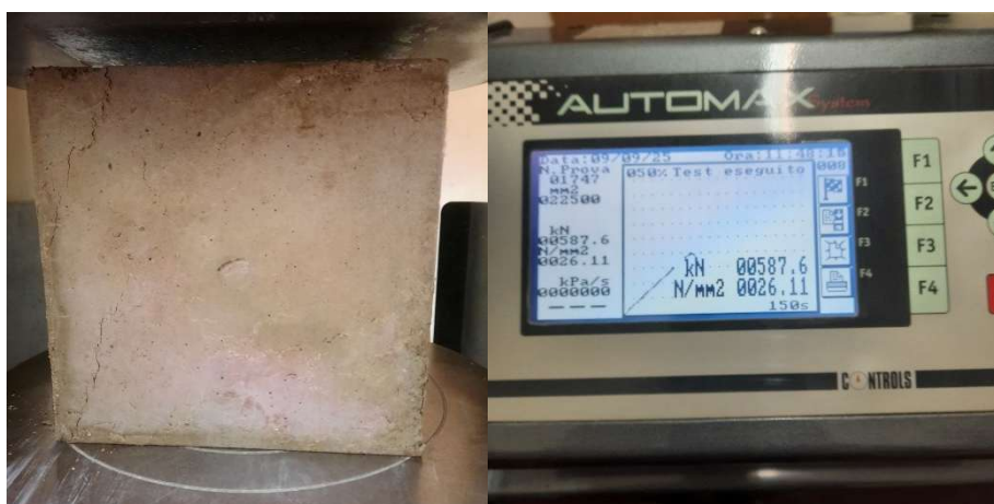
Figure 40. The failure crack pattern of the 120-day specimen.
