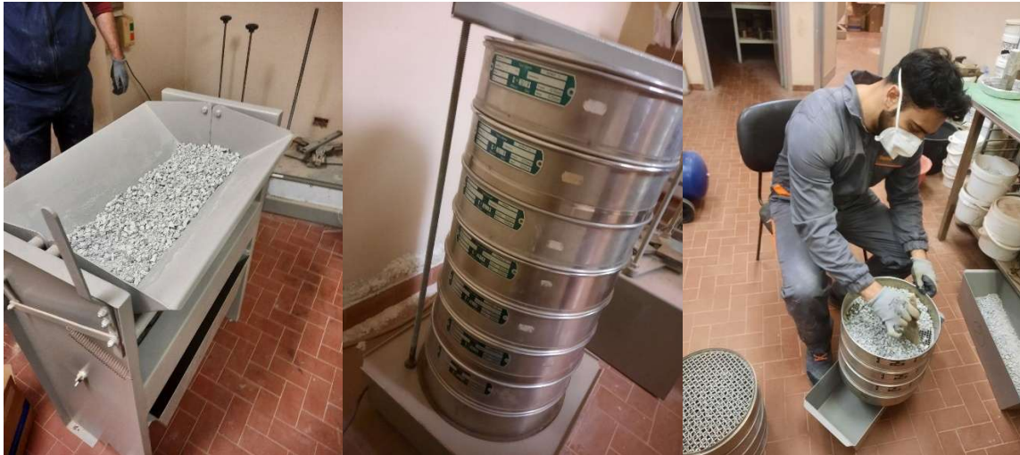
Figure 14. The sieve analysis process which is also called the granulometry test to understand the distribution of the aggregates considering the size and dimensions. The pictures are taken in the laboratory of the university of genoa.
