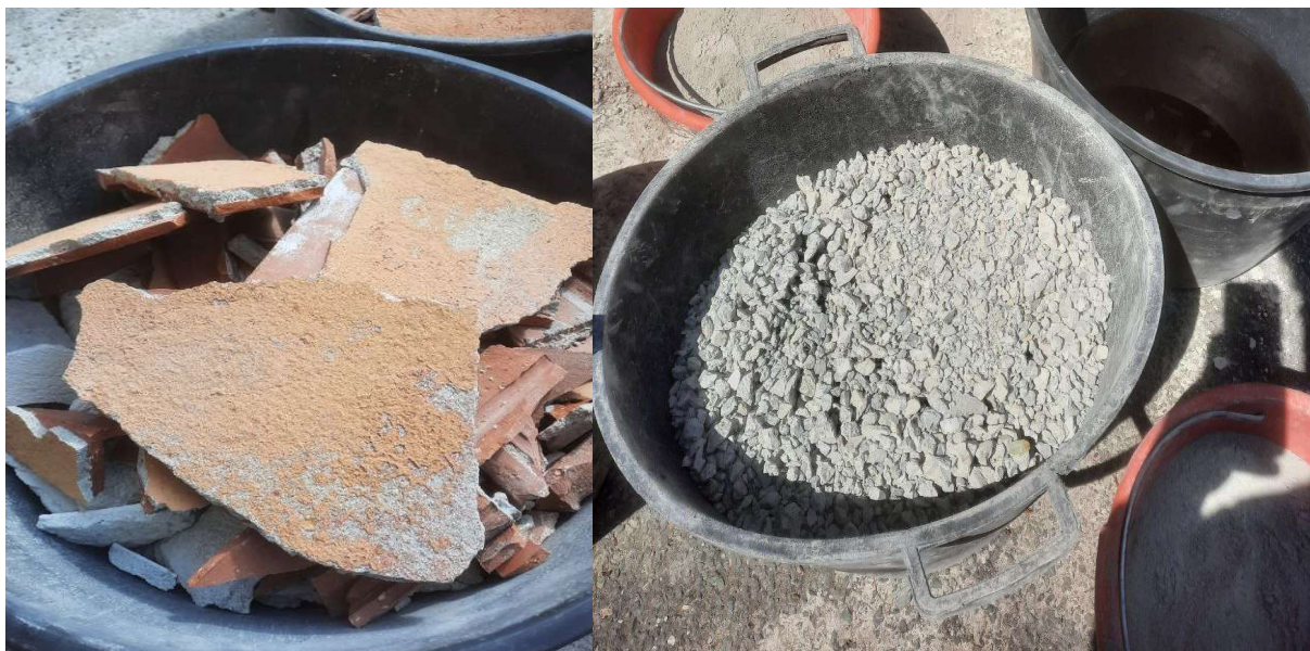
Figure 13. The pictures are taken in the laboratory of university of genoa. on the left it is the mixed debris, on the right is the broken concrete.
