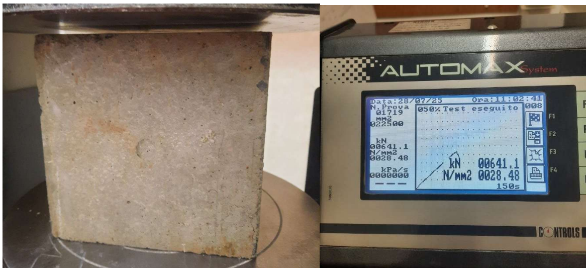
Figure 28. The failure crack pattern of the 90-day specimen.
