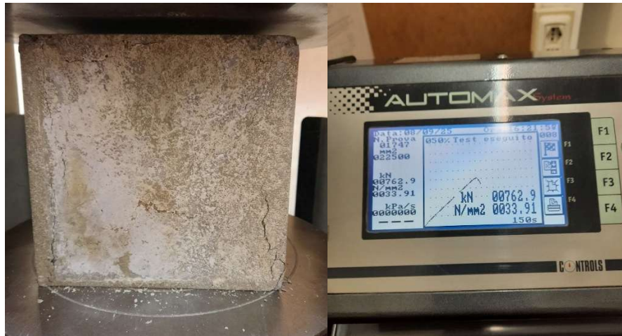
Figure 46. The failure crack pattern of the 90-day specimen.
