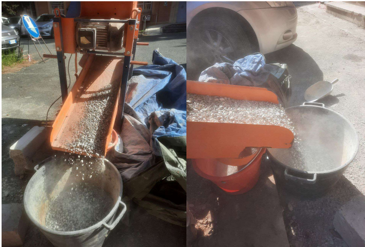
Figure 21. The mini jaw crusher crunchy crushing pieces of debris from the demolition of the buildings into smaller aggregates. The pictures are taken in the laboratory of university of genoa.
