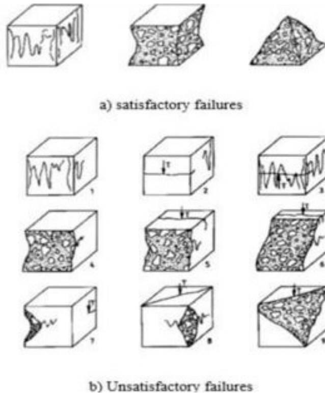
Figure 20. Failure patterns observed in concrete specimens after compressive strength testing. (a) Satisfactory failure characterized by inclined shear cracking and uniform crack distribution, indicating good bonding and homogeneous stress transfer. (b) Unsatisfactory failure showing localized cracking and aggregate–paste debonding, associated with weak interfacial transition zones and non-uniform internal structure.
