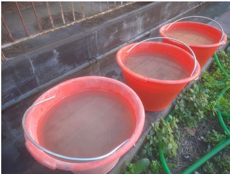
Figure 16. The aggregates are immersed in water for 1 hour
