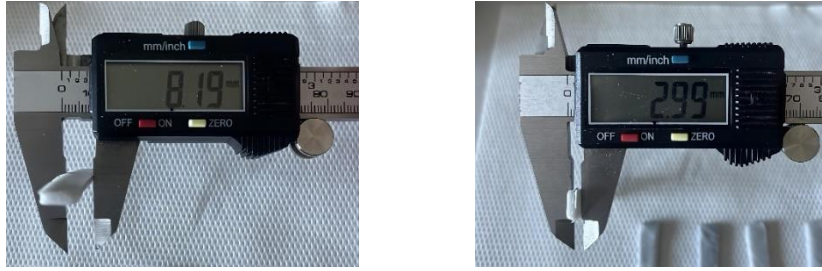
Figure 46: Preliminary dimensional measurement of the 3D-printed rectangular specimens using a digital caliper. The images show the measurement of the specimen thickness and width, parameters necessary for defining the sample cross-section and for the subsequent processing of the mechanical data obtained from the flexural test.
