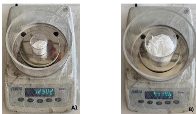
Figure 27: Weighing of the components for the preparation of the PCL-brushite composite. (A) Weighing of \text{Zn}^{2+} -doped brushite, used as the ceramic component of the composite; (B) weighing of polycaprolactone (PCL), used as the polymeric matrix.
