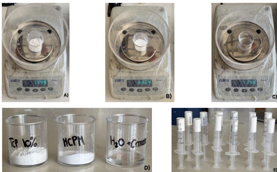
Figure 21: Preparation steps of 10% Zn 2+ -doped brushite cement. The images show the main operations performed for reagent weighing, preparation of the cement mixture, and shaping of the cylindrical samples. In particular: (A) weighing of zinc-doped \beta -tricalcium phosphate ( \beta -TCP:Zn 10%), used in an amount of approximately 7,94 g for each single preparation; (B) weighing of monocalcium phosphate monohydrate (MCPM), used in an amount of 6,30 g; (C) weighing of the distilled water-citrate solution, used as the liquid phase and as a retarder of the setting reaction, in an amount of approximately 4,75 g; (D) weighed reagents placed in their respective containers before mixing; (E) cylindrical samples obtained by inserting the cement paste into previously modified sterile 5 mL syringes.
