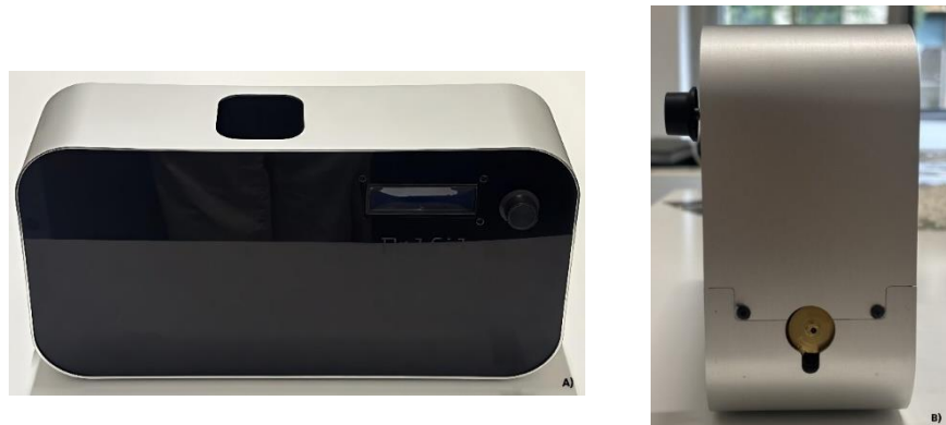
Figure 30: Felfil Evo extruder used for the production of the composite filament. (A) Front view of the instrument, with a display for visualization of the main process parameters, including temperature, screw rotation speed, and electrical absorption; the parameter adjustment knob and the upper hopper for pellet loading are also visible. (B) Side view of the instrument, with particular emphasis on the nozzle through which the filament is extruded.
