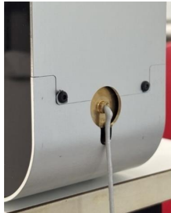
Figure 32: First extrusion trial of the PCL-brushite composite using a 2,85 mm nozzle, performed by setting a temperature of approximately 170 °C. The filament obtained appears macroscopically darker than the filaments produced in the subsequent trials, suggesting a possible effect of excessive thermal treatment on the material.
