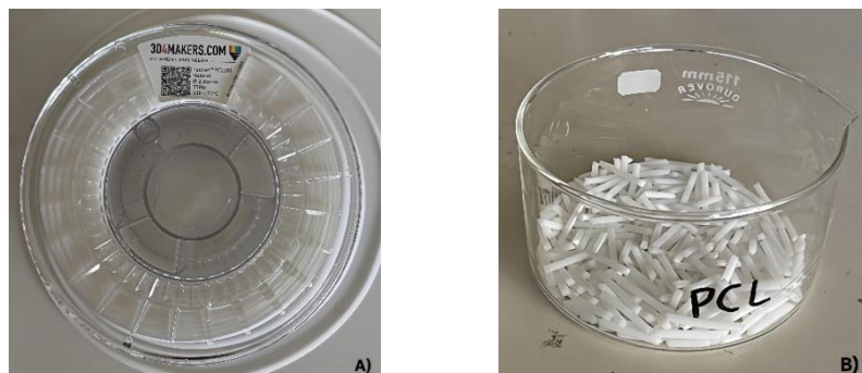
Figure 26: Preliminary preparation of PCL for the fabrication of the PCL-brushite composite. (A) Polycaprolactone (PCL) spool used as the polymeric matrix; (B) PCL cut into small portions in order to promote the subsequent melting of the material and facilitate its mixing with the ceramic component.
