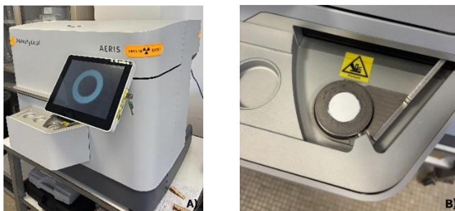
Figure 24: Acquisition of diffractograms by XRD analysis. (A) PANalytical AERIS diffractometer used for the analysis of powder samples; (B) insertion of the mold containing the material into the analysis chamber of the instrument.
