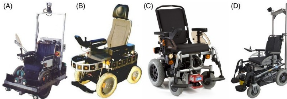
Figure 1.1: Examples of smart wheelchair platforms equipped with sensing and computing units for autonomous navigation and collision avoidance.
