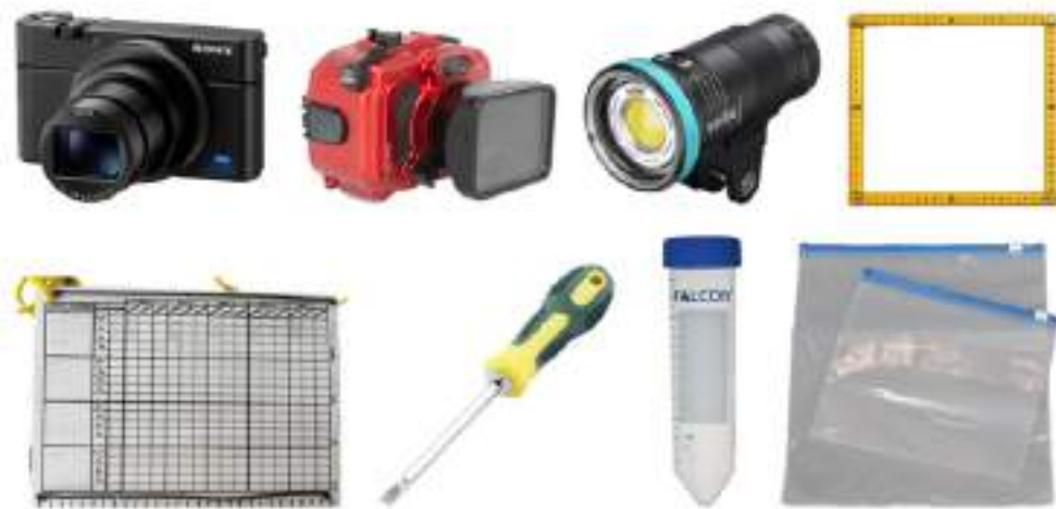
Figure 11: equipment used by diver A in the upper line: from the left: SONY® RX100 MKVII; ISOTTA® diving case; WeeFine® headlight; folding wooden ruler. Equipment used by diver B in the lower line: from the left: scientific PVC slate; Falcon® tubes; plastic zip-lock bags.
