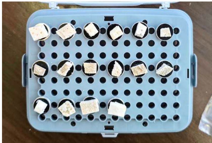
Figure 8 - Quadrangular bone sections mounted on stubs for scanning electron microscopy (SEM).
