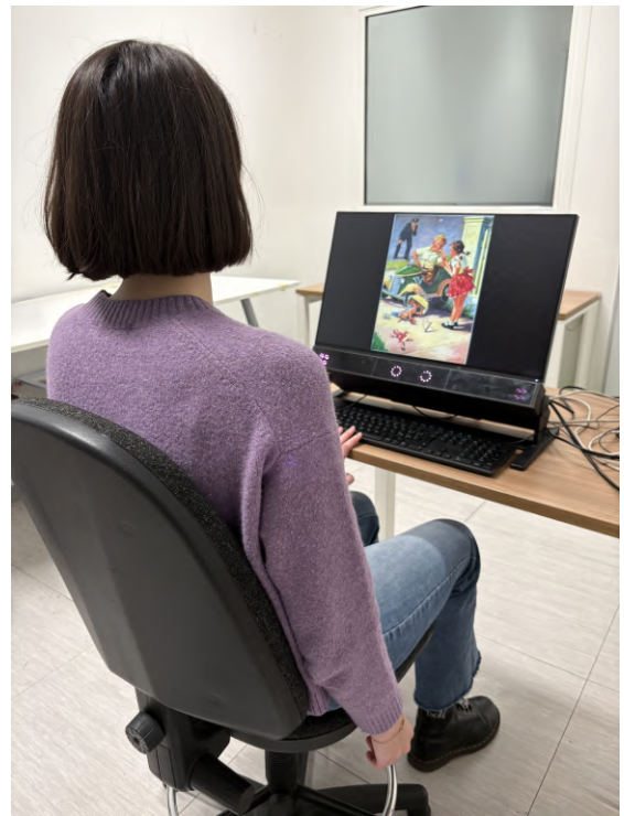
Figure 4.3: Close-up and participant's viewing position of the experimental setup used for the data collection study. The participant is seated in front of the Tobii Pro Spectrum eye tracker and the companion monitor, which displays the stimulus images while gaze data and audio descriptions through a microphone are recorded. The keyboard is used to progress through the experiment timeline.
