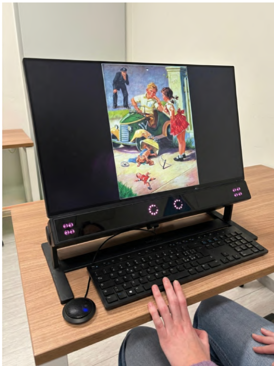
Figure 4.3: Close-up and participant's viewing position of the experimental setup used for the data collection study. The participant is seated in front of the Tobii Pro Spectrum eye tracker and the companion monitor, which displays the stimulus images while gaze data and audio descriptions through a microphone are recorded. The keyboard is used to progress through the experiment timeline.
