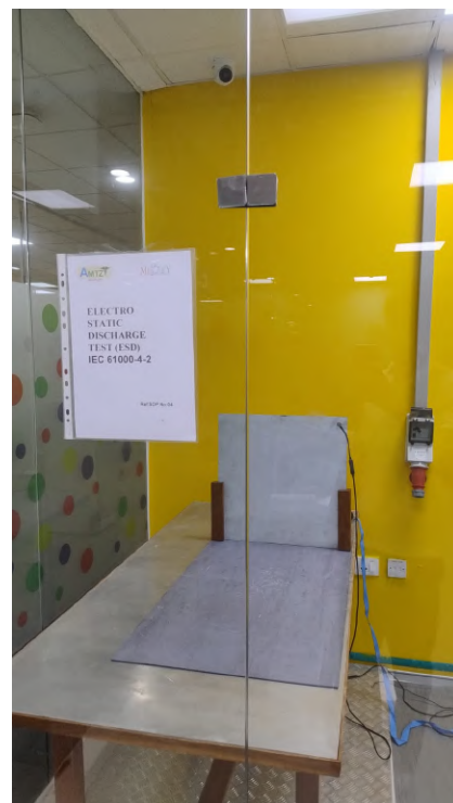
(c) Electrostatic discharge (ESD) testing station.
