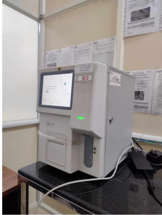
Figure 9.8: KB22 Auto Hematology Analyzer.
