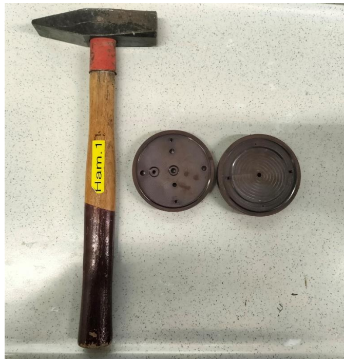
Figure 9 Punching tools and hammer used for Kapton® foils
