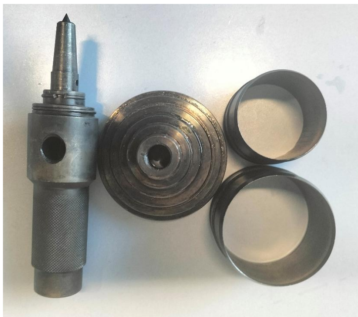
Figure 16 Punching tool: smaller-diameter punch (diameter 40 mm) for electrode cutting and larger-diameter punch (52 mm) for membrane cutting.
