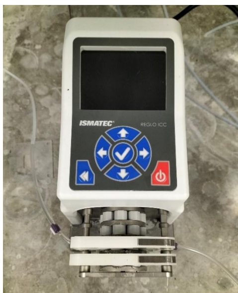
Figure 2 Ismatec Reglo ICC Digital Peristaltic Pump
