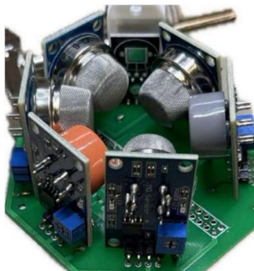
Figure12. Sensors Placement on Manufactured PCB
