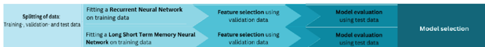
Figure 3.2.1: Flow chart showing the steps and data used during training, model evaluation and model selection
