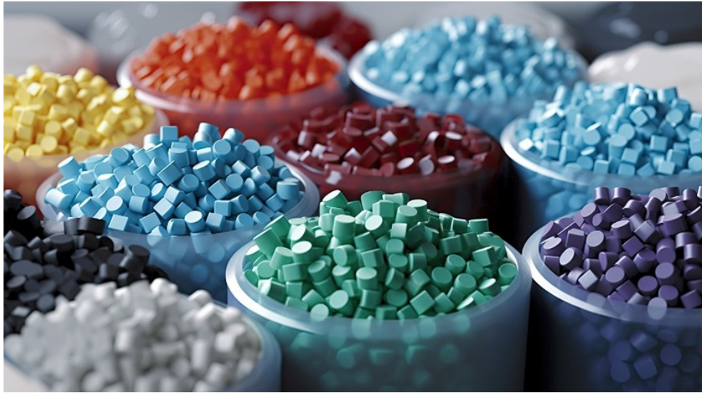
Figure 3.3: Colorful polymer granules sorted by hue, ready for industrial processing and manufacturing applications.
