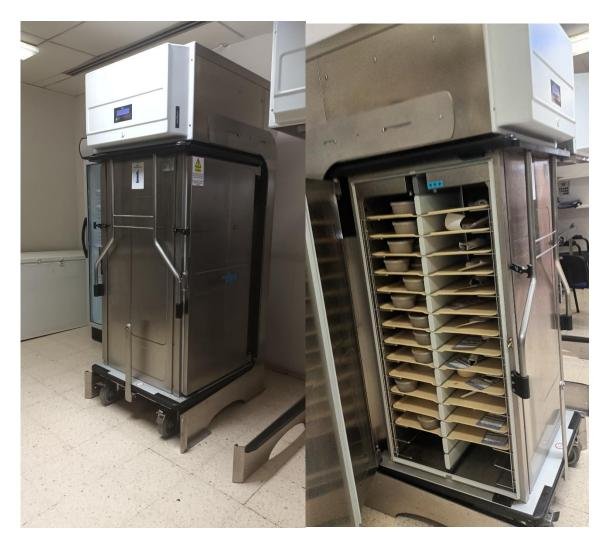
The BPOD contains 12 trays on each side, separated by heat and cold generating areas. Food will be heated for a total of 45 minutes which include
