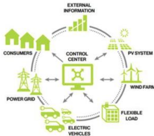
Figure V.2 Virtual Power Plant integration scheme
