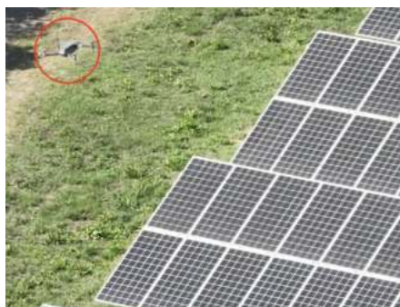
Figure 1.1: Picture of a drone inspecting a PV plant taken during a test in Predosa (AL).
