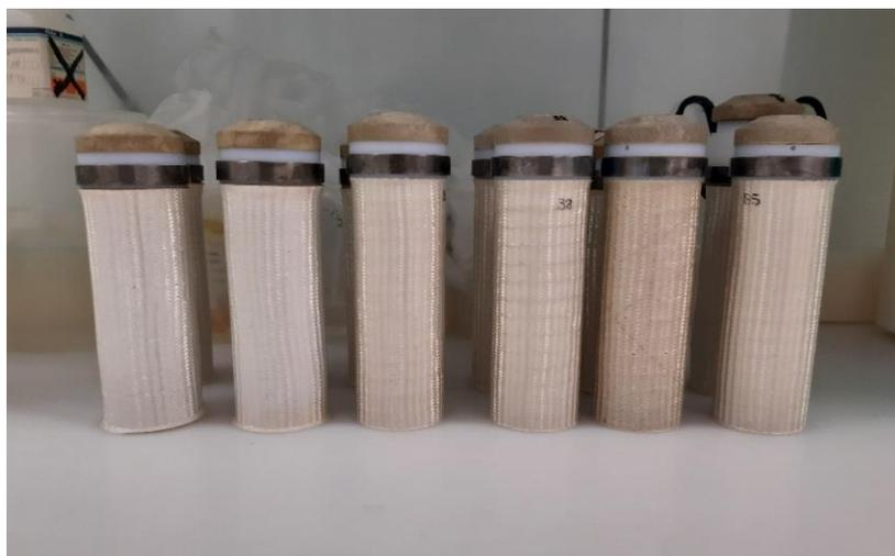
**Figura 4.6** Vessel in Teflon<sup>®</sup> "XP-1500 plus"
