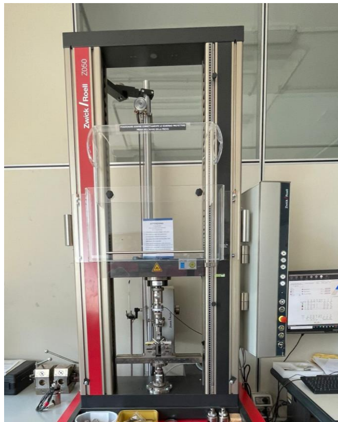
Fig.8. Zwick/Roell Z50 universal machine for mechanical test used to conduct mechanical bending tests.
