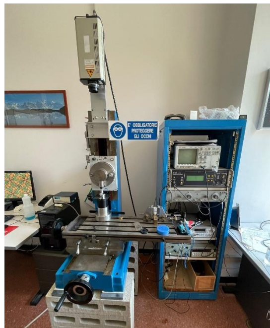
Fig.6. Prototype for DMA used to conduct analysis on specimens.
