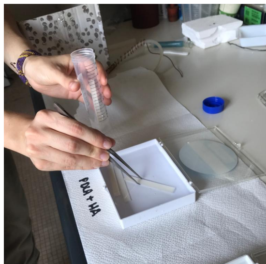
Fig.5. Extraction of the specimen and placing in sterile plastic test tubes.
