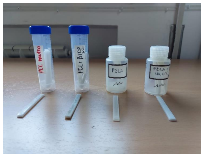
Fig.3. Specimens printed following ISO 178 standard, in order: neutral PCL, PCL/ \beta -TCP, neutral PLLA and PDLA/HAP.
